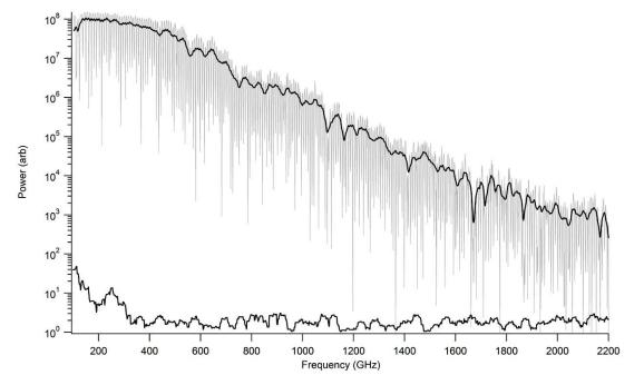
Air at 1 ATM with water vapor (below). No processing was performed because head spacing was adjusted to remove interference fringes from the region of interest.
